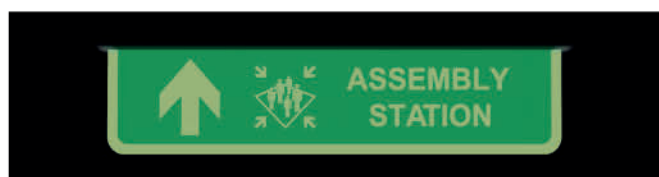
After power loss (3 hours, 22 mcd/m 2 )
